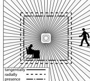
Reliable presence detection largely depends on the number, condition and arrangement of the lens segments. The IR Quattro with its square detection zone of 49 m<sup>2</sup> divided up into 13 levels and 1760 switching zones senses the smallest of movements. With
