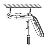
This luminaire is a class II, non-maintained emergency luminaire and only requires mains active and neutral wiring. Close the top cover after mains wiring.
